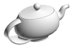
Let's start by making the handle surface a Solid with the **Make Solid** command.
