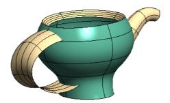
We'll use a **Pipe Surface** to make a spout, but we need a curve to define the path of the surface.
