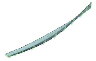
That's a thin net of control points. Let's try increasing the control points in the U direction first.
