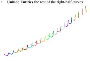
Now we'll use the Fit Curve command again to fit all the curves at once. We'll use the same settings we used for the single curve.
