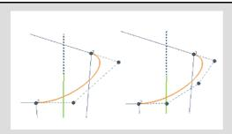
Start Modify Curve Control Points, select middle control point and move from p1 to p2.
