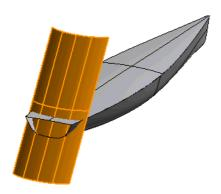
We'll start by using the Make Solid command to obtain a single solid hull.
