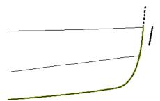
That flat bow won't be very fast since it's flat in the front, so we'll need to create a rounded surface there. Let's make another **Connect Curve** curve with the other line to get an idea of the type of rounded surface we are looking to create for our bow.
