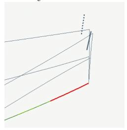
Now we'll create the first **Connect Curve** curve between the dashed line and the boundary curve. We'll use this curve to trim the hull surfaces.
