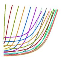
Now let's create a **Lofted Surface** surface from these curves. New surface will interpolate the curves exactly.
