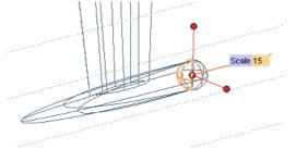
Now let's make a solid from these two surfaces and **Solid Union** the two keel solids to the hull.
