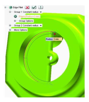
Now fillet the inside continuous edge at a value of R3. We need to rotate the model using **Pan Zoom Rotate** for the selection.
