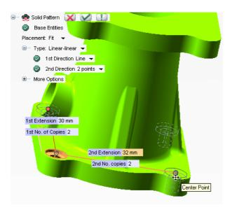
The Pattern Solid has been created. Rebuild the model.
