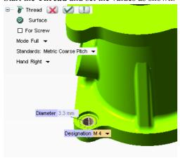
The **Hole** and **Thread** is created at one corner of the base solid.
