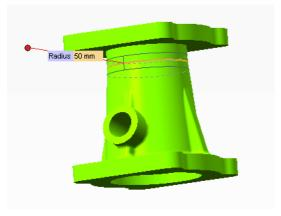
From 2007.1 version, a new feature called the **Fillet Face-to-Face** has been introduced. By using this command it is possible to apply a constant radius fillet by selecting two faces. Let's use this command and create a fillet now.
