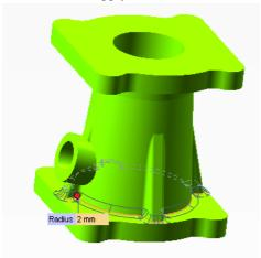
Apply a fillet of Radius1mm to the bottom edge of the boss.
