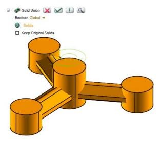
Now, we should add fillet to all the chamfer edges as well as the other edges of the three Arms.
