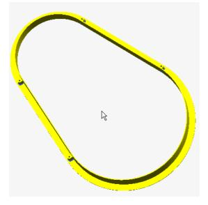
As we review the part, it becomes obvious that it could sure use another boss for a bolt that's located half way around between the bosses we just added. There does not appear to be any good geometry available to snap the boss' location to, so we shall use a slightly different method for positioning and orienting this boss we're adding.
