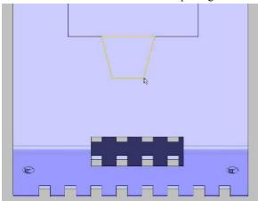
• Insert a new blind slot of Depth 1mm, Radius 0.5 on side and base and 0.1 on ../../Common as shown.
