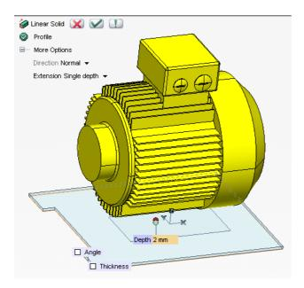
• Click ✓ OK to create the first face of the Sheet Metal casing.
