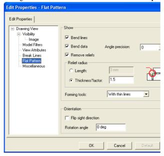
Under the Flat Pattern tab you can control the visibility of the Bend lines and Bend data by checking/unchecking the boxes.
