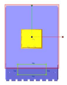
• Insert a new blind slot and set the depth to 20mm
