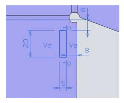
• Make a slot with the profile and make it Thru all as shown
