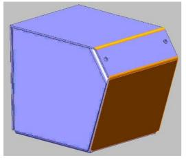
You can see from the image below that the **Unbend** occurs only at the specified portion of the Motor casing. This is a "local" unbend.
