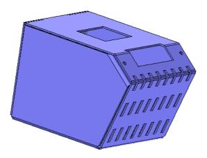
• Move the Work Plane on to the top flange and add one more profile on the flange as shown.
