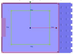
• Click on Smart Object Library and click on Insert Smart object and select PUNCH CONIC selecting rectangular profile corners as placing points.
