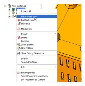
ThinkDesign will automatically open a **New Drawing** with the "flat pattern" View of the selected Sheet Metal part. The image below shows our casing in its **Flat Pattern View**.
