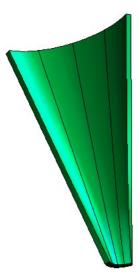
You can see that this solid has Profiles that are twisted along the height of the model.
