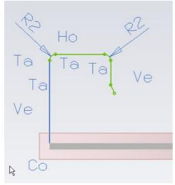
Let us now create an **Extruded Flange** with the sketched profile running through the chain of edges of the top face of the solid.
