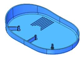
Select Tools Modeling Check Manifold. Now the model is manifold solid.
