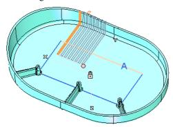
Here is the result. Analysing the object, the slots weaken the rigidity of plastic model. We need to strengthen their shape.
