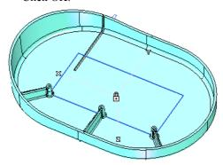
Use the **Pattern Solid** to pattern the new slot with the values of 1st Extension30 and 1st No. Copies8 as shown in the image below.
