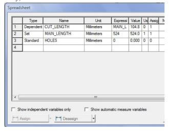
Click on Unit - Millimeters box and select Scalar from the box.
