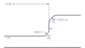
Profiles define the shape of solids, and every protrusion or a slot uses a profile to define its shape. Here is the cool part: if you change a profile, the associated solid or feature changes, too! You have been creating profiles all along, you just may not have known it. Every time you selected lines and arcs for a **Linear Protrusion** or a **Linear Slot**, ThinkDesign turned them into a profile.
