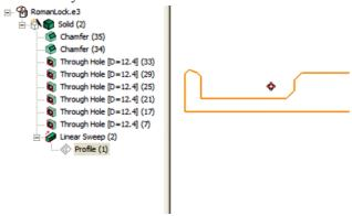
You cannot select individual lines because ThinkDesign combines all the lines into a single profile object. So, if a profile is a single object, how do we modify the individual lines?
