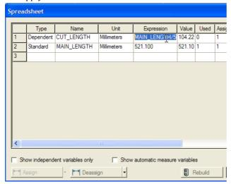
Double click on CUT\_LENGTH. The value field has been grayed out. This indicates that dimension is linked.
