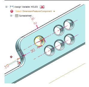
In the next step let's see how we can activate/deactivate hole feature using **Spreadsheet** only.
