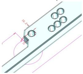
For your information: Hitting VOK or Enter when you are changing the driving dimensions records the changes to the value, but does not update the model. This allows you to change several values prior to rebuilding. This change was painless, but complex models can take longer to rebuild.
