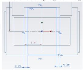
Again we captured design intent. We could have just as easily defined the width of the cut and made it symmetric about the centerline using a width/half-width pair. By dimensioning the extensions instead we guarantee that no matter how wide the clevis is, the extensions will be 0.25 inches from the inside surface.
