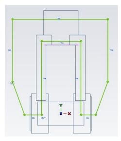
Add a coincident constraint as shown in the image below to lock the profile to the solid.
