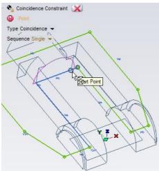
Add the remaining geometric constraints to control the shape.
