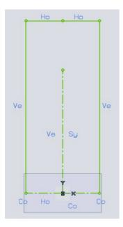
Add geometric constraints to the profile starting with a **Ground Constraint**.
