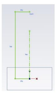
Create a similar Profile on the other side of the Reference line, with some arbitrary values of length and Width. Since the profile is Symmetric, we can apply the Symmetric Constraint to complete the Rectangle.
