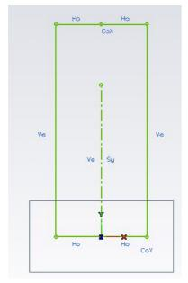
Use Make Reference to convert the Bottom Horizontal lines as Reference Geometry.
