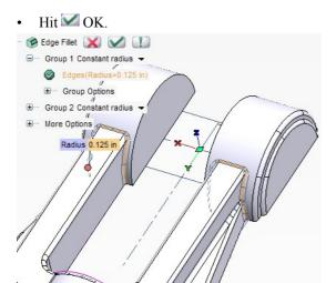
We finished half the part. Remember that the order that we add features determines the result. It's time to mirror it and then join with the copy to create one solid.
