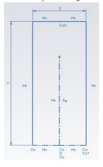
The profile will not be fully constrained because the centerline has one end point that is not constrained. It is not important that we do so, and it does not matter because we can still create a solid from a partially constrained profile. That's what we shall do in the next step.
