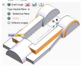
The angle is slight but if we were to zoom in, we would notice the difference. Had we applied draft before we created the main boss, the boss would be pointed at a 2 degree angle below the horizontal. We would not want that. Next we will add fillets.
