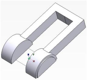
We shall need to rotate the Work Plane because we want to create a profile so that the sweep direction is along the horizontal reference line.
