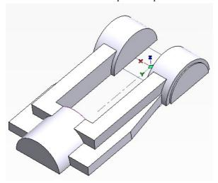
Add draft to the non-mating surfaces that are perpendicular to the parting plane.
