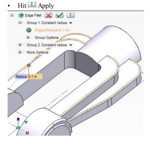
Now fillet the pair of edges in between the previous edges. We could not fillet these edges until we filleted the ones before hand. Otherwise the blend where the webbing meets the secondary boss would have been bad.
