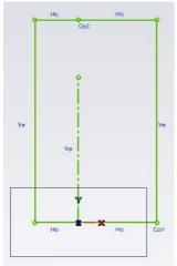
Apply the **Symmetry Constraint** between the Curves on the either side of the Reference Line as shown below. Select the Curves on the left hand side of the Reference line as First Group and Curves on the Right Hand side as Second Group and Reference line as the Axis.
