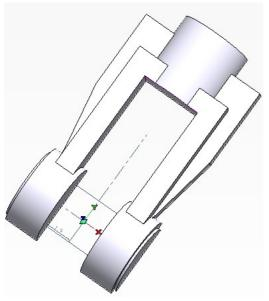
Unhide the necessary profiles, position the work plane, and then duplicate the half-moon profile.
