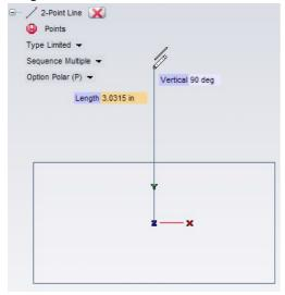
Use Make Reference to convert the line into reference geometry.
