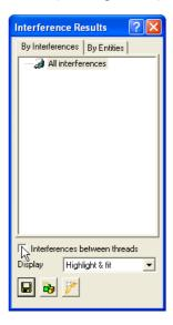
No interferences are found between the Screw's threads and the Housing component when the  $\overline{\mathbb{Z}}$  Interferences between threads box is checked OFF.
