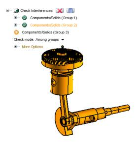
Click calculator button in the Selection List to start the interference checking. Notice the result shown below:
