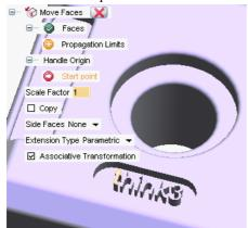
• Click on Propagated limits and select the top face of the solid as shown in the image below.
