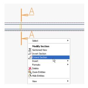
• Click to place the top and bottom ends of the cutting plane line a little closer to the view.
