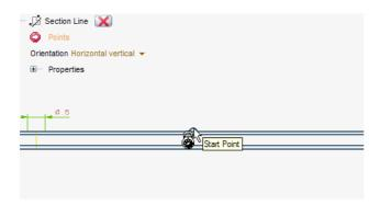
• Snap to the End Point directly under the first point on the lower edge of the view to define the line.
