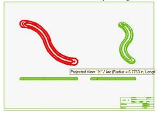
The Tooltip shows the name of the view according to how it was created, and the properties of the entity. In this standard top view, it shows the Projected View named "b" and the entity we were over.
