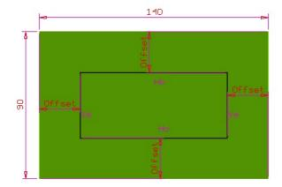
• Draw lines of 20mm length at the corners of the rectangle at angles of 45/-45 and 135/-135 degrees, respectively (see image below for reference). Be sure to use the **Intersection Point Snap** tool.
