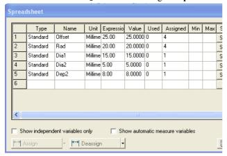
Let's assign the same name - Dia1 - to all of the larger hole diameter dimensions, using the Assign button in the Spreadsheet form:
