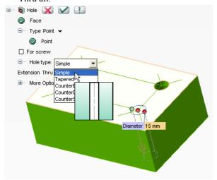
• Create eight holes - again using **Hole** - of **5** mm Dia. at the end points of the angular lines. Make their Extension Blind, and set the Depth8. See image below for reference.
