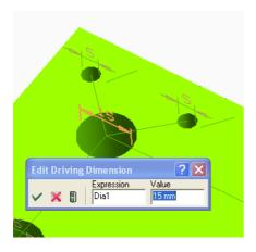
Do the same for one of the smaller hole diameter dimensions, and the depth. Call them Dia2 and Dep2, respectively:
