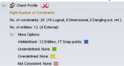
• Apply these same constraint conditions to the other 3 corners of the rectangle. Use the **Check Profile** periodically to see the constraint status of the Profile.
