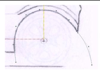
• Use Insert Curve through Control Points command to sketch the remaining curves in this view.
