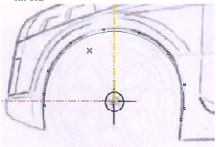
• Start **Modify Curve Control Points** and select the curve. Drag and move the control points, change the curvature to obtain the better shape as shown below.
