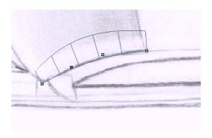
Select one or two control points and move the curve to match the curvature of the windshield and also to give it a better internal continuity.
