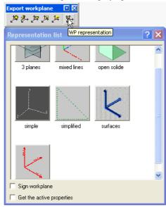
Click on the WP representation button (fourth) on the Workplane manager toolbar to get the Representation list. (If you're not able to locate this toolbar, go to **Tools** Customize and select it under the Toolbars tab.) Double click on the mixed lines option to insert the reference lines.
