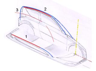
The two new curves can be joined using the **Connect Curve** command or by using the **Two D to Three D Curve** command and selecting the connect curves of the front and rear curves.
