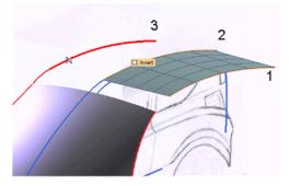
Applying the **Lofted Surface** command we got the geometry that shows the windscreen and the roof as shown in the image below.
