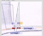
Try to change the U values or the Weight values by dragging the pointers or inserting numbers in the Mini-Dialogs.
