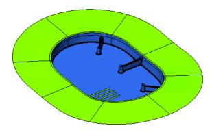
We need to identify all the edges that are required to define the parting plane.
