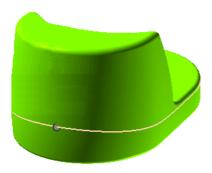
The previous command shows a cuspid point between two curves and now using **Curve Continuity** we want to reduce this.
