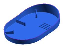
We need to identify all the edges that are required to define the parting plane.
