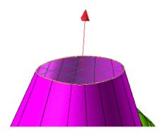
Changing the parameters on the Linear surfaces, redefining the feature, will have an automatic update of planar linked surface.
