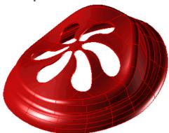
We will add some vent holes in the cover. We'll use a profile from another layer and then use the **Linear Slot** command to create the vent.
