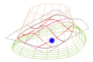
Use again **Trim Surface with Limits** where as Limits is the splitted Skin and the Surfaces are the four draft linear Skins. Keep the bottom sides.
