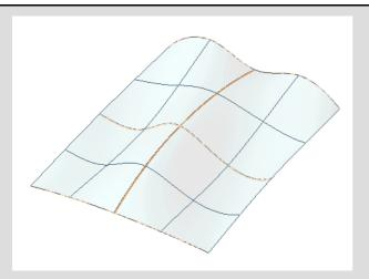
By Spined Surface, be careful while modifying the control point not to snap to the existing model geometry. The curve MUST stay parallel to the work plane!! By snapping to other geometry the curve will no longer be on the same work plane and the original command that created the shape will no longer work.
