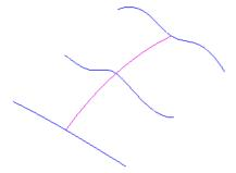
The base surfaces are all set. Next we need to create some surfaces for a cover. We will create the first surface using the **Lofted Surface**, **Spined Surface** or Global Sweep command. Let's prefer now Global Sweep because will be the better mode if you need, next time, to change completly the inner sections.
