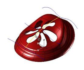
We changed the work plane location because the curve editing process has to be parallel to the plane where lies the curve.
