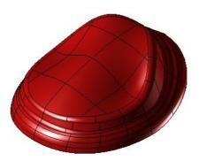
In this step we'll use the completed surfaces and turn them into an open solid using the Make Solid command.
