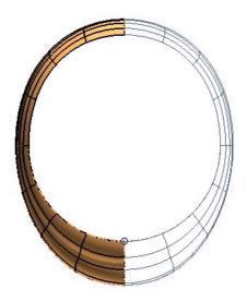
If we take a look at the front view, we can see that the surfaces aren't perfectly tangent; we haven't impose it before. So we'll use the **Surface Continuity** command to fix that.
