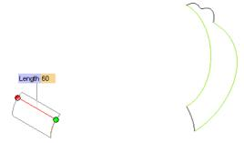
Now we will connect (blend) these two surfaces together using the **Connect Surface** command but this command isn't associative. So will use the **Connect Lofted Surface** that permits it. This command makes the connect surface tangent to the two other surfaces. By using the construction surface to aid in tangency creation, the model will remain tangent when it is mirrored later.
