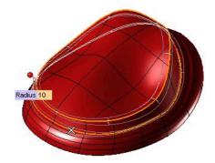
The model is shaping up, but what is a solid without thickness? Let's use the Solid Shell command to fix that.
