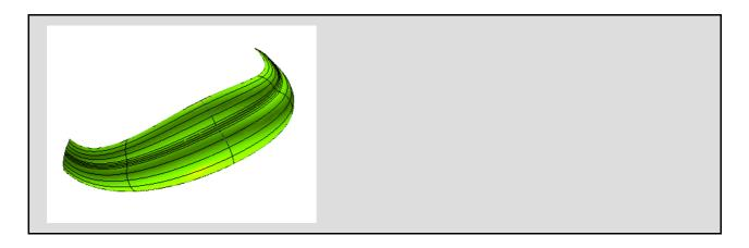
The base surfaces are all set. Next we need to create a couple of surfaces for a cover. The first surface we'll create using the **Linear Surface** command.
