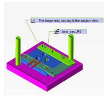
This gives the JrD a quick view of the Annotations attached to the Die block holes.
