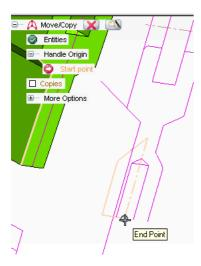
• Pick the intersection of the centerline and the baseline of the original profile to move the geometry to the End Point.
