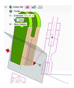
The slot on the back of the part is the same as the one we just cut. Instead of cutting a second slot, we'll use **Mirror Solid** for this one. That way, if we ever change the first slot, the mirrored copy will change, too.
