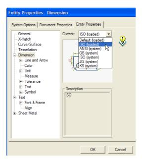
Dimensions are special entities. Using "Entity Properties" on Dimensions, it is possible to set the "Style", like appearance, dimension colors, dimension orientation and position, arrowheads, units of measure, and text height.
