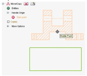
• For the <sup>©</sup> End Point snap to the mid point of the upper horizontal line of the rectangle, as shown below.
