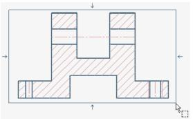
• After selecting the view, ThinkDesign will place the start point of the handle in an arbitrary place. To move the handle origin; in the selection list, right click on the Start Point and select Reset, then snap to the mid point of the horizontal line of the section view as shown.
